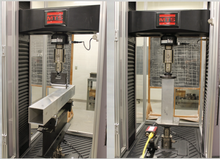
Set-up for axial and side crush experiments.
