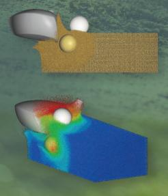
The velocity for the sand can displayed as a fringe plot and it is also possible to blank part of the soil to better visualize the impact on the structural parts embedded in the soil.
