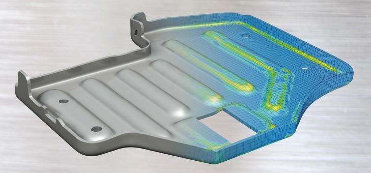
Accurate modeling that captures forming defects leads to fewer prototype runs in the tool shop, improved productivity and higher manufacturing efficiency.
