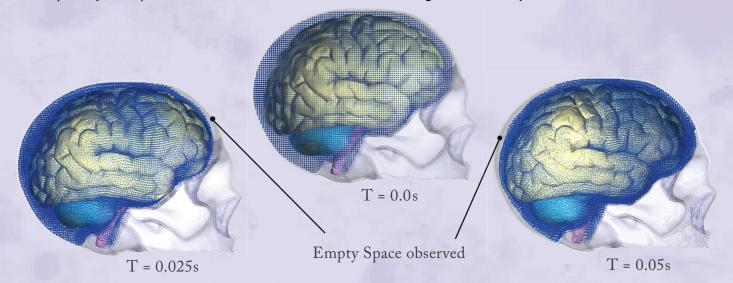
During the rapid acceleration, the fluid particles can be seen to concentrate at the back of the head, thus preventing the brain from going backward relative to the skull. Under the rapid deceleration, the fluid particles are then concentrated at the frontal lobe, again preventing the brain from moving forward and thus stopping it from impacting the skull. Hence, demonstrating the dumping effect of the cerebrospinal fluid.
