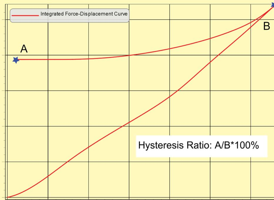
The curve as a result of integrating the force versus displacement curve. This curve is used to find “the internal hysteresis ratio” which is done based on the values of A and B as listed in the graph.
