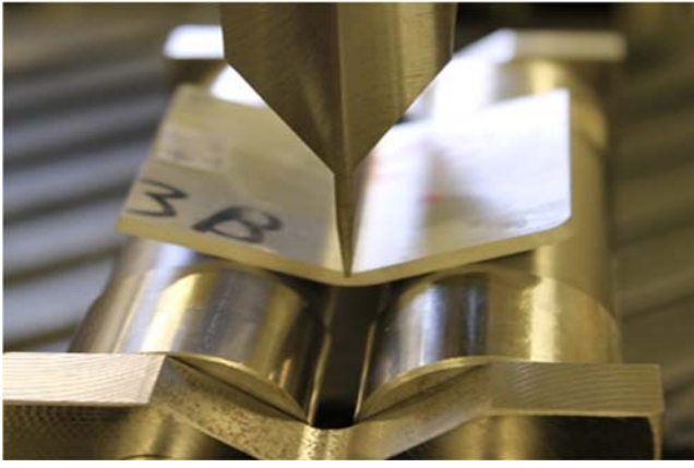
Figure 1. VDA 238-100 plate bending test setup.
