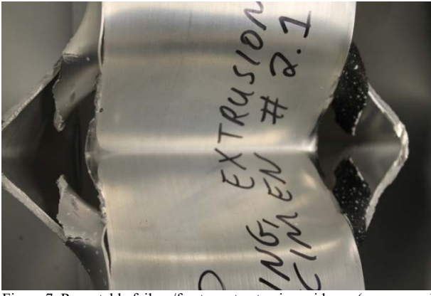
Figure 7. Repeatable failure/fracture at extrusion midspan (compressed surface in contact with midspan roller).
