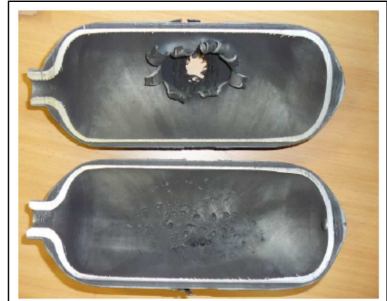
Figure 5. Perforation of tank with large mushrooming for trial with water #HE0208
