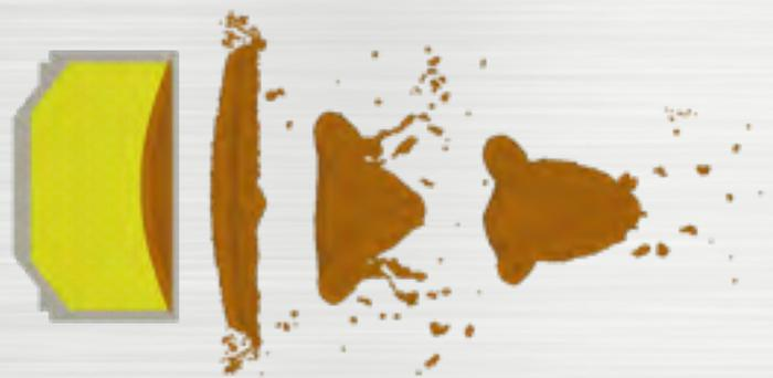
Figure 3: IMPETUS Results: Development of the EFP's forming phase. Half model shown to increase visibility.
