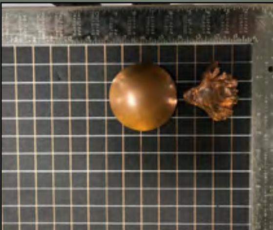
Figure 2: An example of an initial Liner and the resulting EFP. Items are from Rock Mechanics and Explosives Research Center, Missouri S&T [Jensen, 2019].
