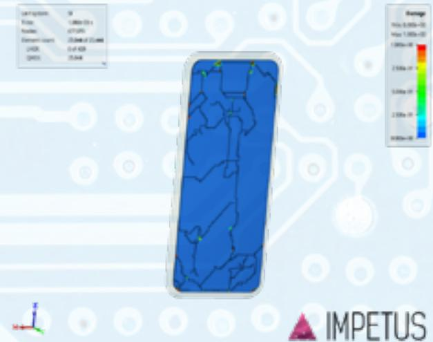
Figure 2 shows the crack propagation after impact.
