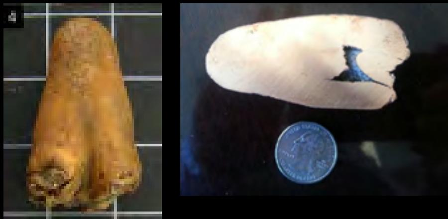
Figure 2: The original flyer plate geometry (a), the projectile from an EFP (b) and the cross-section highlighting the material deformation (c).
